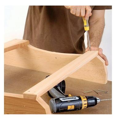
Begin the seat assembly by screwing the lower back rail to the seat sides with one screw at either end of the rail. Then you will want to add **slat number 4** as seen on the drawing with a single screw at either end.
